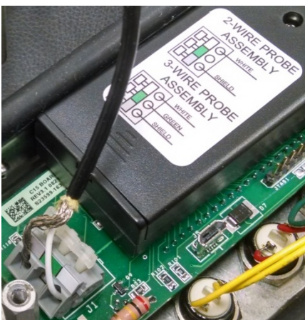
Figure 1: Probe Assembly Lead Attachment
